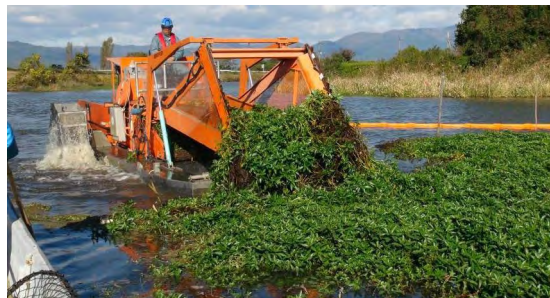
Figure 5. A workboat called “aquatic weed harvester” usually used for collecting submerged weeds.
